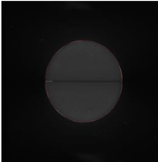
Figure 13. Fit using an ellipse. The ellipse fitting package supplied by OpenCV can only fit a whole ellipse so we mirror the shockwave over its bottom edge. The ellipse's major and minor radii are used to describe the dimensions of the shockwave.
