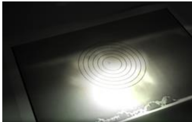
Figure 2. An example of a frame of a film being projected onto the grid of a Kodograph.
